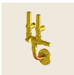
Double safety valve To protect the refrigerant circuits against high-pressure. A single valve is fitted in the factory. The double valve means you can switch to a second valve without having to drain the refrigerant circuit for maintenance operations. Model: DSV
